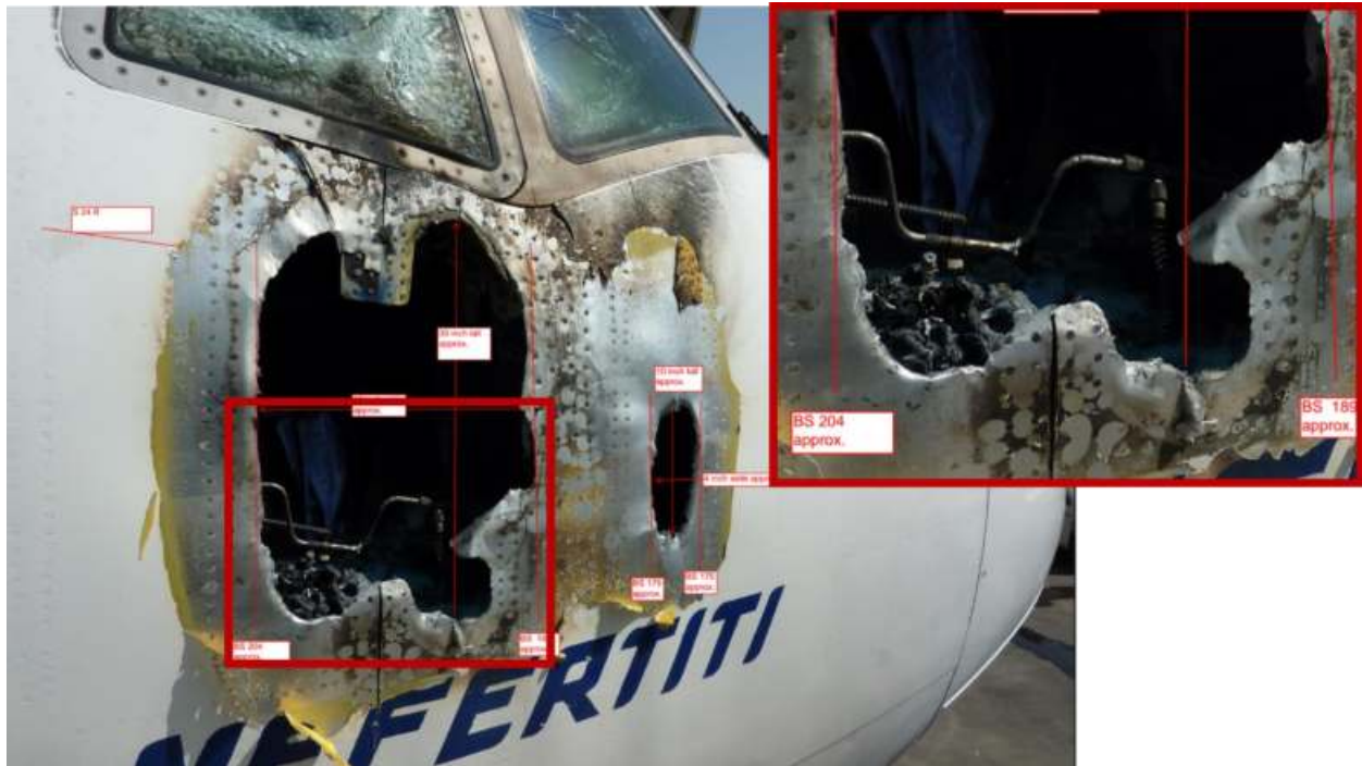
Photograph 2 Damage to forward starboard fuselage of EgyptAir B777 registration SU-GBP, at Cairo International Airport, 29 July 2011.
