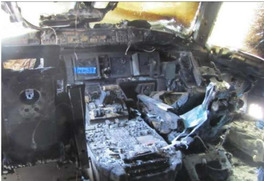
Photograph 1 Damage to flight deck of EgyptAir B777 registration SU-GBP, at Cairo International Airport, 29 July 2011.
